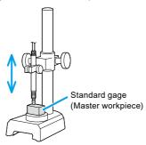
5 In ABS mode, bring the pointer of the meter close to zero.
