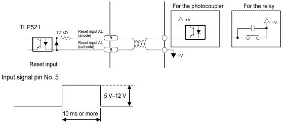
• To apply 12 V or more, add a resistor externally.
