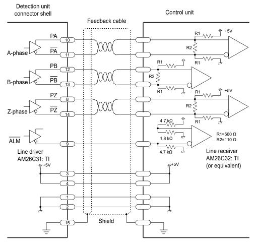
To use the square wave output signals, connect the output signal cable as shown in the figure below.
