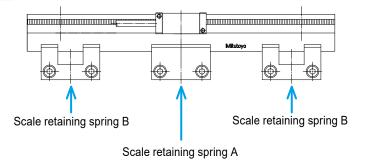
**2** Temporarily fix the main scale with the scale retaining spring B.
