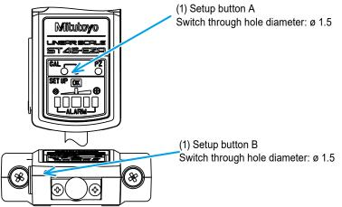
2 Adjust the moire direction of the Detector so that the signal strength judgment results in "OK" on the setup indicator.
