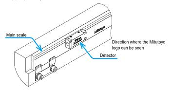
• Put the serial number sticker near the location where the scale is mounted on the machine for the main scale with the effective length of 10 mm–80 mm.
