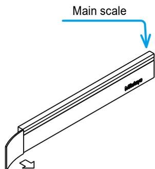
Peel the scale protection tape.
