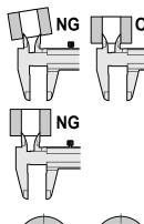
• For inner diameter measurement, bring the inside measuring surfaces into close contact, and read the display when it is maximum: a direct line between the measuring surfaces passes through the center of the cross-section.
