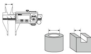
Insert the inside measuring jaws as deeply as possible into the workpiece.
