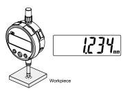
Gradually and lightly place the contact point on the workpiece in the same orientation and conditions as for reference point setting, and then read the indicated value.
