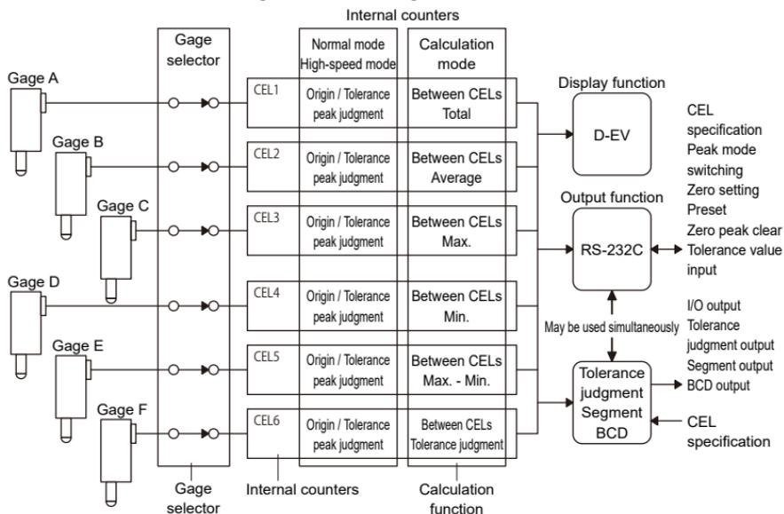
Consider which data to output from the I/O connector, and each CEL mode can be selected by changing the setting of the I/O function mode (parameter no.22). For details, see ["5.3 I/O Connector Terminal Function"](#) (page 47).
