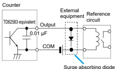
Output withstand voltage: Max. 24 V
