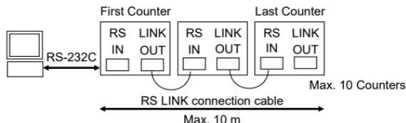
When the D-EV is connected as shown below, the D-EV displays the data of the EV Counter A.
