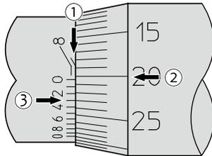
For "0.20 mm" in ②, read the location where the reference line on the sleeve meets the graduation line on the thimble.
