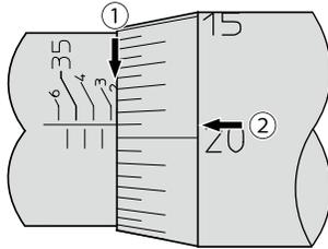
For "0.195 mm" in ②, read the location where the reference line on the sleeve meets the graduation line on the thimble.
