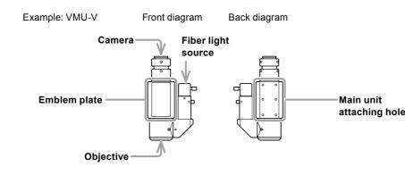
Tips The front side of the main body has main unit attaching holes (six threaded holes, M4, 0.7 pitch, 6 mm depth) to mount the main body on a device that are the same as on the back side. An emblem plate is affixed to the front side of the main body as shown in the diagram above. To mount a device on the front side, remove the emblem plate and secure it on the back side of the main body.
