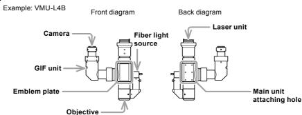
The front side of the main body has main unit attaching holes (6 threaded holes, M4, 0.7 pitch, Tips 6 mm depth) to mount the main body on a device that are the same as on the back side. An emblem plate is affixed to the front side of the main body as shown in the diagram above. To mount a device on the front side, remove the emblem plate and secure it on the back side of the main body.
