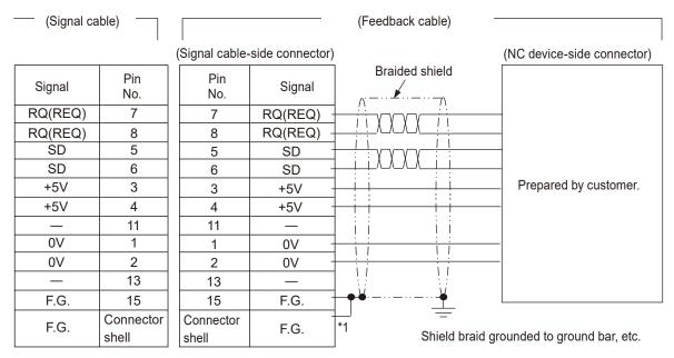
\*1: If a shielded drain wire is present, connect it to pin 15 of the D sub-connector.
