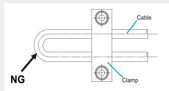
• If a cable is subject to repeated bending, allow it to move freely without fastening it, and take care to prevent application of stress at the point where the cable is clamped near its end.
