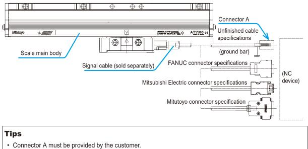
• The customer is responsible for wiring connector A and ground bar connection.
