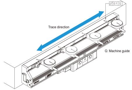
E Positioning can be simplified by using a base point, such as a positioning pin, as shown in "2.6 Precautions Regarding Mounting Surface Design" on page 28, but the mounting position must be confirmed.
