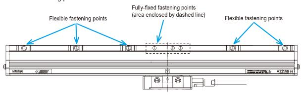
· Flexible fastening points when fastened
