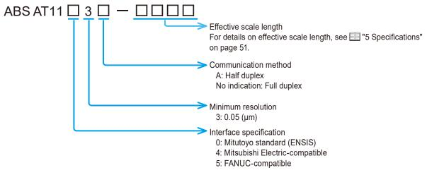
• Interface specification: Model number of applicable system and scale unit
