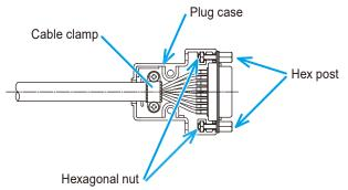
**3** Put the other half of the plug case in place, secure it with the plug case fixing screws (M2.6 x 14 and hex nuts), and finally securely tighten the hex posts.
