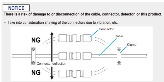
• Care should be taken to avoid extreme bending or pulling at the base of the signal cable during the entire stroke range.
