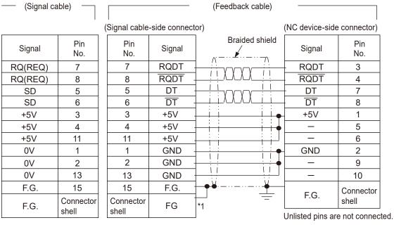
Shield braid grounded to ground bar, etc.
