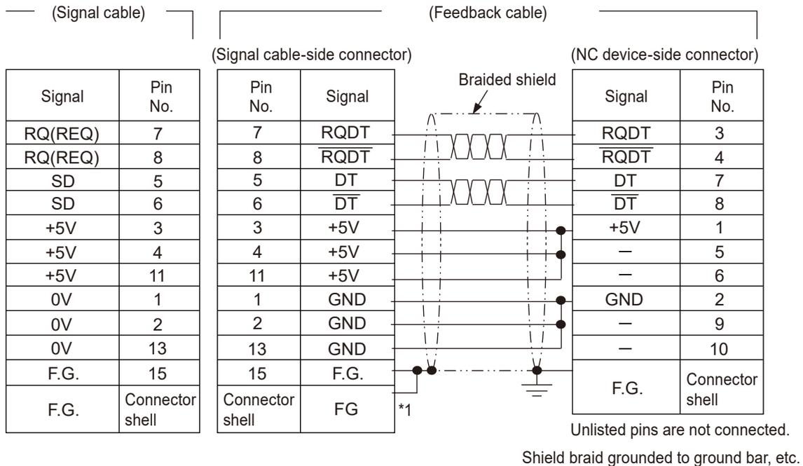
\*1: If a shielded drain wire is present, connect it to pin 15 of the D sub-connector.
