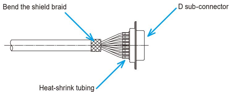
**5 Set the D sub-connector in the plug case.**
