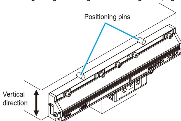
**3 Securely fasten the scale main body to the scale mounting surface of the machine body.**
