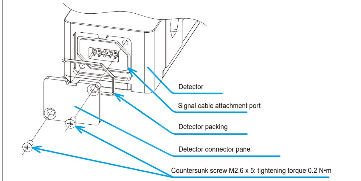
**3 Connect the signal cable to the detector.**
