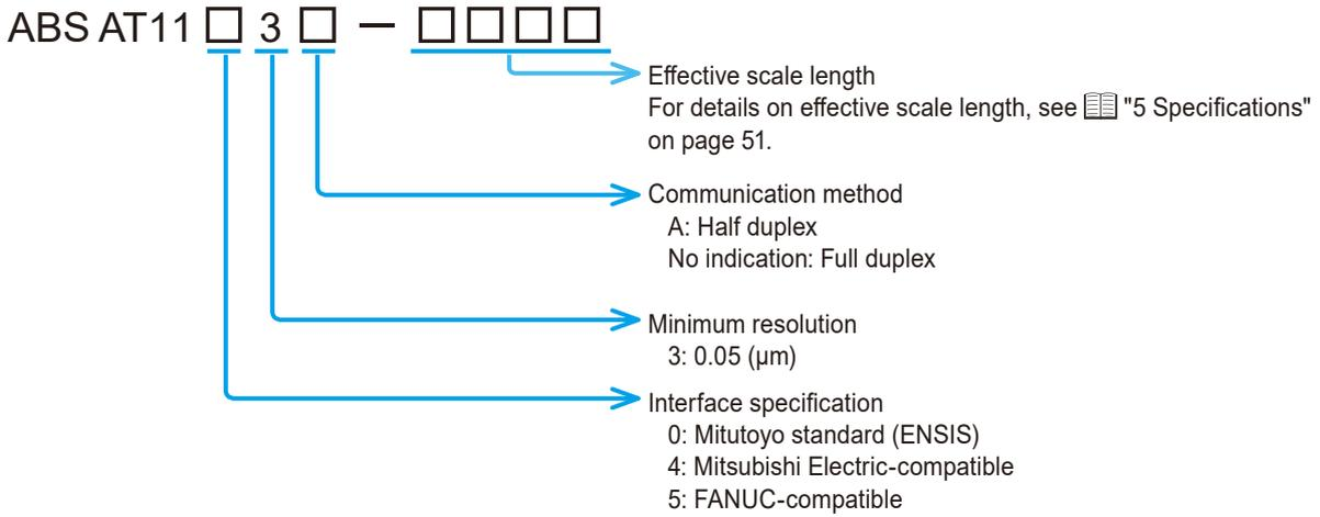
● Interface specification: Model number of applicable system and scale unit
