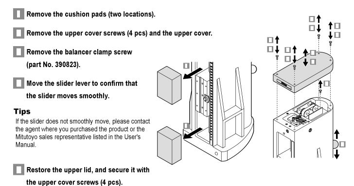
Store the removed balancer clamp screw so that it does not get lost. This screw is necessary when transporting the product for repair or for major relocations.
