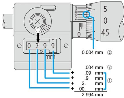
For "0.004 mm" in ②, read the location where the vernier graduation line meets the graduation line on the thimble.
