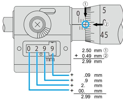
For "0.49 mm" in ②, read the location where the reference line on the sleeve meets the graduation line on the thimble. This is normally read up to a graduation of 0.01 mm (as shown in the figure above). However, it is also possible to visually read up to a graduation of 0.001 mm (as shown in the figure below).
