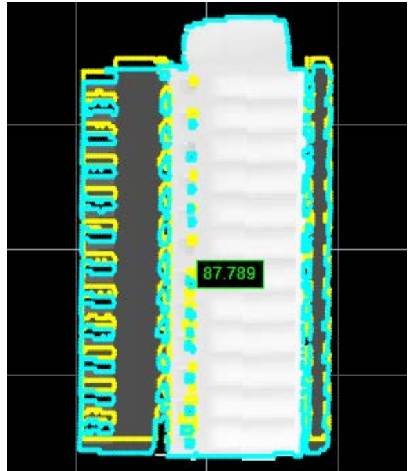
Edge points along top of model removed. Part is accepted. (Min set to 85%.)
