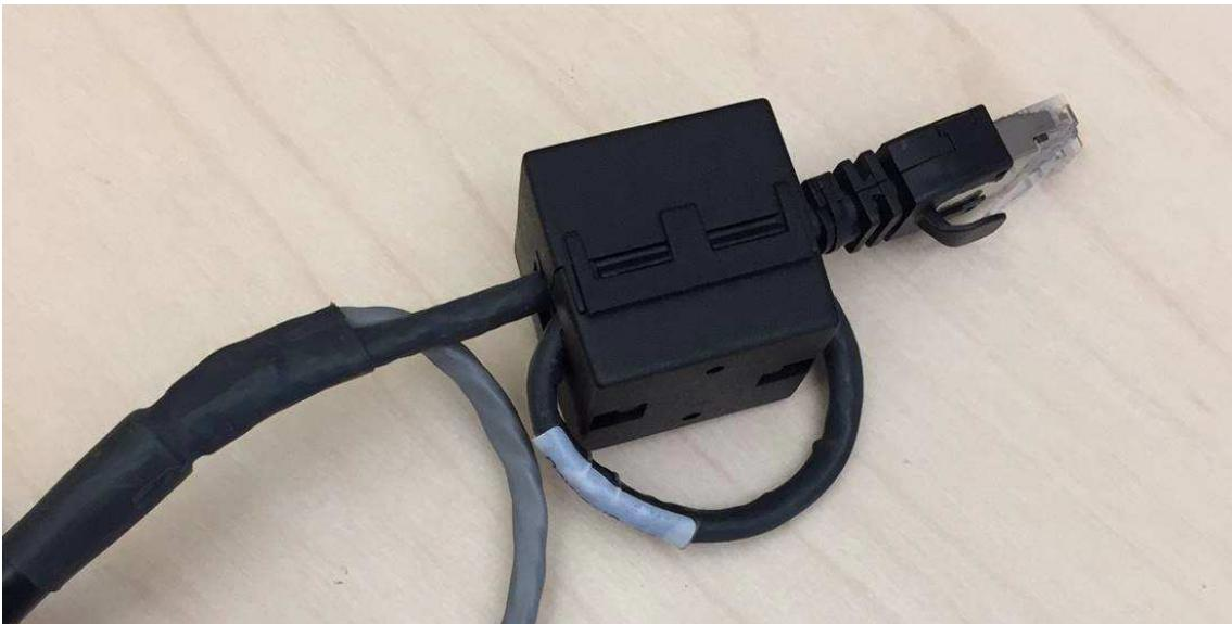
If high frequency noise is present in the power line, looping the SM1008S power cable through ferrite core assists in reducing the noise. The ferrite core should only have the power part of the cable looped inside, and not the Ethernet part as the ferrite core could interfere with Ethernet data transmission.
