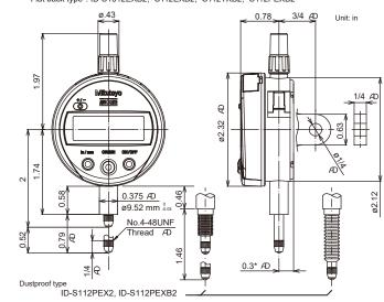
AD This is the symbol of American Gage Design (AGD). It means that this type conforms to appropriate dimensions of Dial Indicators in ASME/AGD 2 and has interchangeability.
