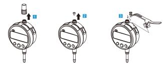
Rotate the cap counterclockwise to remove it from the product.
