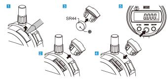
1 Use a flathead screwdriver or similar to remove the battery holder.
