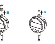
1 Rotate the cap counterclockwise to remove it from the product.
