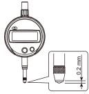
A rubber damper is attached to this product to soften the plunger impact. Although the indicated value may not be stable at the bottom dead center due to the elasticity of the damper, this is not a malfunction.
