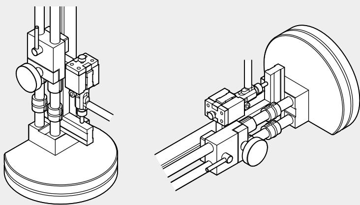
As an example, the following explanation describes the procedure for using this product in a vertical orientation with a Dial Indicator.
