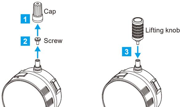
**1** Rotate the cap counterclockwise to remove it from the product.
