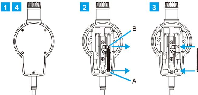
**1** Remove the five screws on the back using a #0 Phillips screwdriver, and then remove the flat back.
