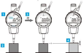
1 Confirm that the product is in incremental measurement (INC display is turned on).
