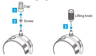
1 Rotate the cap counterclockwise to remove it from the product.
