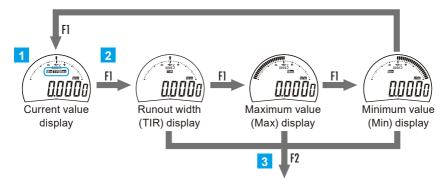
1 Make sure that the measurement mode is set to peak detection (peak detection display is lit).
