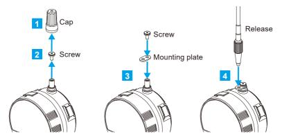
1 Rotate the cap counterclockwise to remove it from the product.
