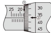
Read the thimble at the location where the sleeve reference line matches the graduation line on the thimble.
