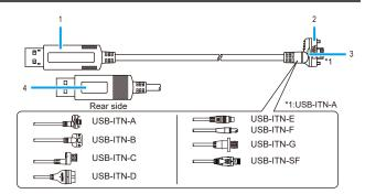
USB connector ("A" plug) Connects to the USB port of a PC or commercially-available USB hub.
