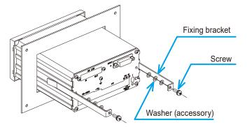
3 Insert the counter main body from the front side of the panel.
