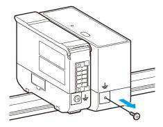
2 Pass the removed terminal screw through the hole in the ground wire's ring lug, and then loosely fasten the lug to the ground terminal.
