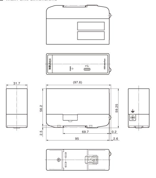
■ DIN rail and connector installation dimensional drawing
