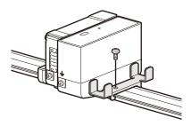
4 Repeat step 1 through 3 to attach the other fixing bracket also to the side with the terminal unit.
