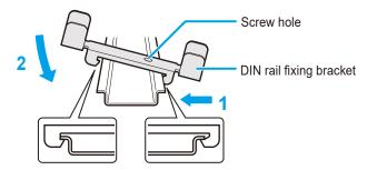
2 Slide the fixing bracket along the DIN rail to where it comes in contact with this product.
