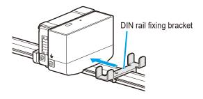
3 Fasten the fixing bracket in place by threading the screw provided with the fixing bracket into the screw hole in the bracket, and then tightening the screw so that it presses against the DIN rail, immobilizing the fixing bracket.
