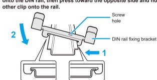
2 Slide the fixing bracket onto the DIN rail to where it comes in contact with this product, and then fasten the fixing bracket in place by threading the screw provided with the fixing bracket into the screw hole in the bracket, and then tightening the screw so that it presses against the DIN rail.
