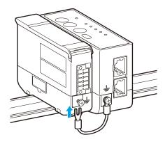
4 Firmly tighten the ground terminal screws on this product and the EJ Counter.
