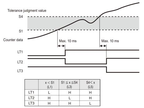
\* With 3-step tolerance judgment, L2 and L4 are not used. (Fixed to 0)
