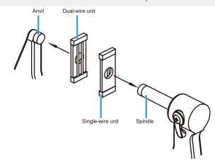
2 Bring the wires into contact with the workpiece (screw) as shown below.
