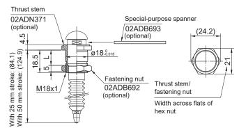
L: base thickness, use the base with a thickness of 10 mm to 13 mm.
