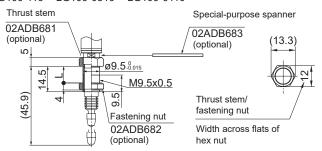
L: base thickness, use the base with a thickness of 6 mm to 10.5 mm.
