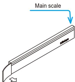
Peel the scale protection tape.
