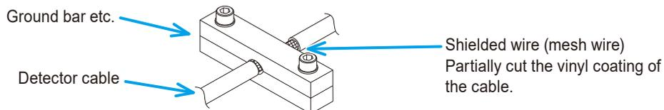
Example: Drawing of using a ground bar
