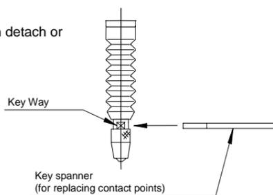
**2) Replacing the rubber boot**
