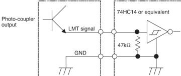
LMT signal receiver circuit
