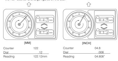
(b) When shifting the slider downwards from the reference surface (B), take the readings from the BOTTOM counter and the small figures on the dial.
