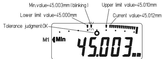
If the tolerance limits are set, the analog bar also shows the upper/lower values. Therefore the state of the diameter to the tolerance limit can be checked easily. The example on the left shows a measurement result of a workpiece, the minimum value = 45.003mm(current value=45.012mm), with the setting of the upper limit=45.010mm and the lower limit=30.000mm
