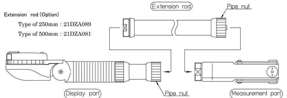
When a deep bore is to be measured, the Digimatic Bore Gage can be extended by the use of the Ex.-rod. Set the Ex.-rod in the following steps.
