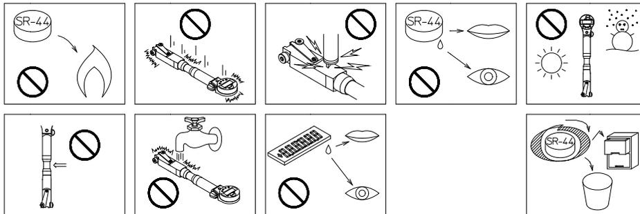
Observe the following precautions to avoid instrument failure and malfunction
