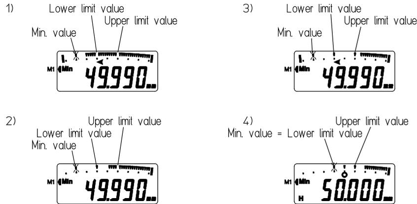
The example as stated above shows a measurement result, the minimum value=49.990mm (No.4) =50.000mm), setting the upper limit=50.010mm, lower limit=50.000mm.
