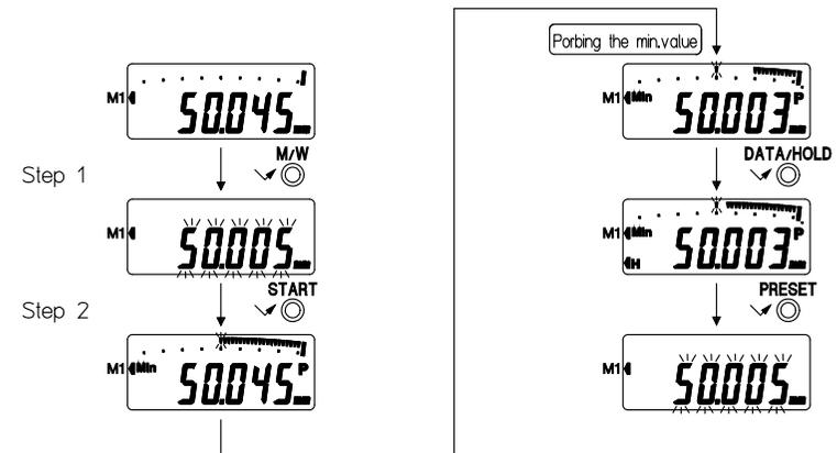
If the master No. is changed, it requires re-calibration of this instrument using the master ring.
