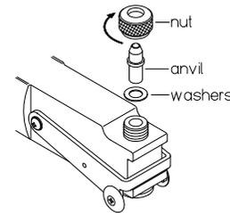
For the required measuring dimension select the appropriate interchangeable washers and the anvil and set them on the main unit. If performing measurement with the interchangeable washers, and the anvil assembled, use a minimum number for each.
