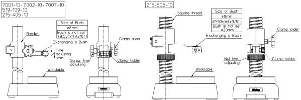
\* Work table 7001-10, 7002-10, 7007-10, and 519-109-10 can be exchanged with accessory work table. Recommended clamping torque for exchanging is 80N cm as to maintain the flatness.
