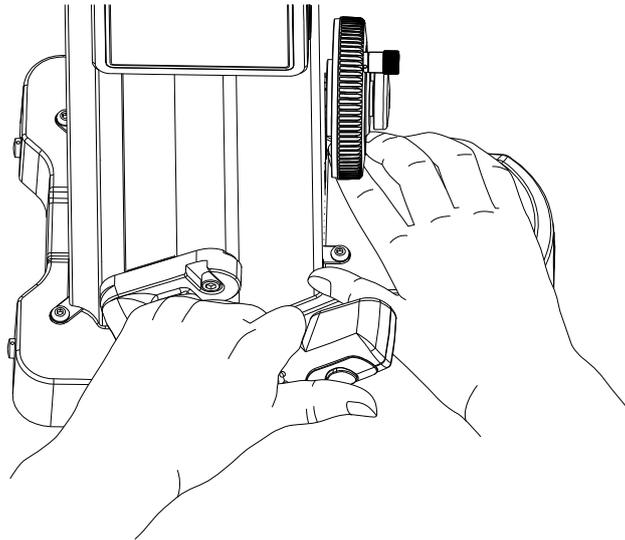
For QMH-600B/QMH-350B/QMH-24"B/QMH-14"B, pressing the air-float switch on the tip of the carrier grip causes air to make the main unit float, allowing you to move it smoothly above the surface plate.
