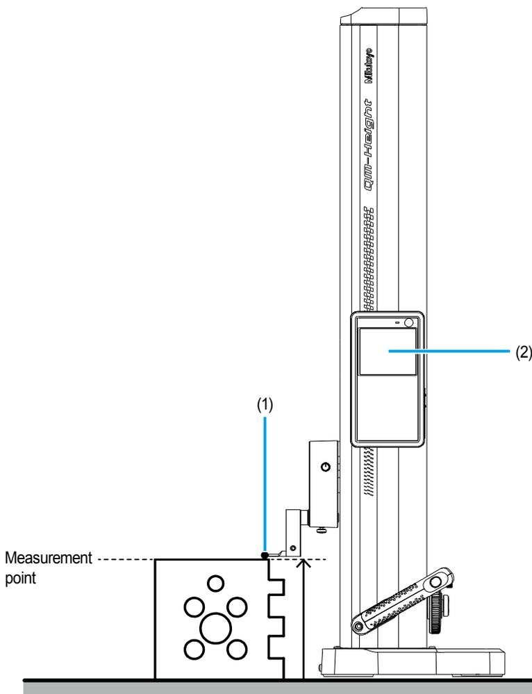
Bring the probe into contact with the point you want to measure (1), and read the displayed measurement (2).
