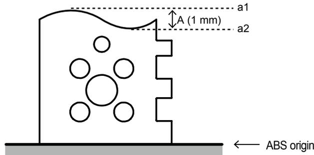
**NOTE** Measure within a range of about 1 mm from the starting point. Measuring with a wider range may increase measurement errors.
