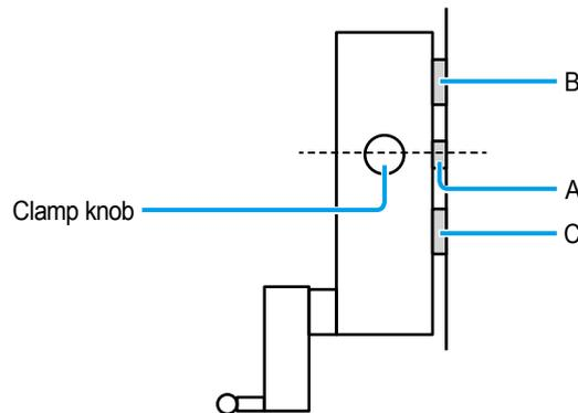
If metal fitting A is not in the center, turn the clamp knob left, and move metal fitting A vertically into the center. From this position, turn the clamp knob right as far as possible, and then turn it left about 5 rotations. The hold function will be released, and measurements can be made again.
