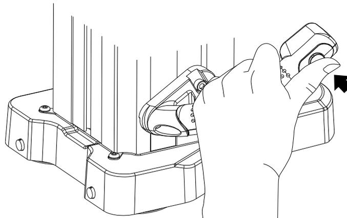
**NOTE** Do not move the product by grabbing parts other than the base or carrier grip. Doing so can negatively affect measurement accuracy and the product itself.
