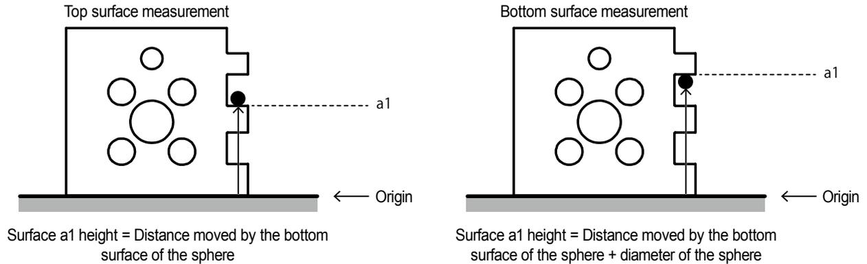
The diameter of the sphere must be set in advance. The following procedure explains how to measure the diameter of the sphere using the provided ball diameter calibration block. This procedure is necessary if you are using the product for the first time or if you are replacing the probe.
