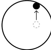
**NOTE** Bring the probe into contact within 0.5 mm of the highest point. Measuring with a wider range may increase measurement errors.
