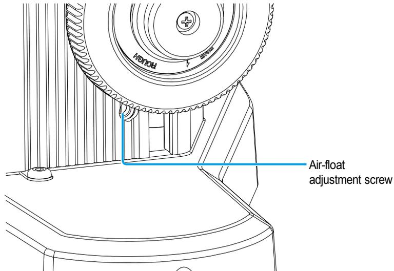
The airflow has been adjusted to provide optimal performance before shipment. We recommend using the default settings as much as possible.
