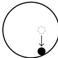
**NOTE** Bring the probe into contact within 0.5 mm of the lowest point. Measuring with a wider range may increase measurement errors.
