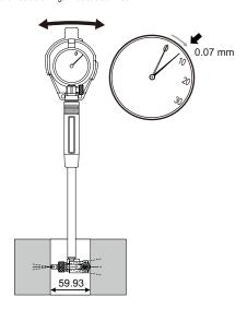
Calculate the measured value by adding the read value (difference) to the dimension of the reference gage.
