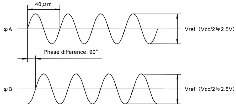
\* If the alarm reset input is specified for the I/F box, the sine waves are not outputted.
