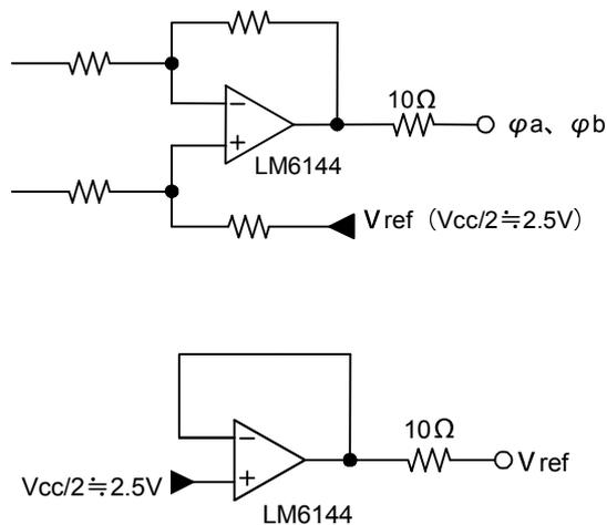
Recommended output circuits of main signal sine wave (phase-A, phase-B)
