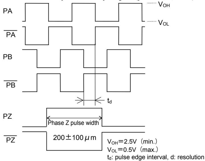
**NOTE** There is no relationship with the phase difference between the PZ signal and PA signal (or PB signal).
