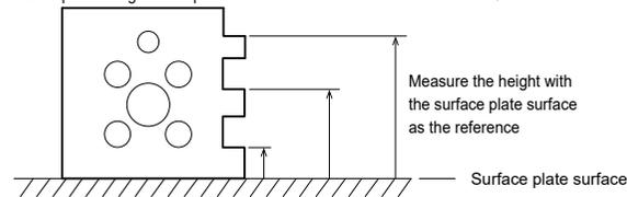
As an example, this section describes how to set the surface plate surface as the reference.
