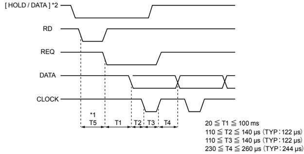
\*1: The time until the [HOLD/DATA] switch goes to the Low level and REQUEST is input.
