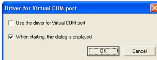
If the [Use the driver for Virtual COM port] check box is turning off, the driver for direct USB is used.
