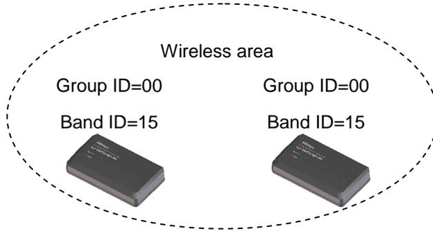
If two or more U-WAVE-R to which same group ID and band ID are set are detected in the same wireless area, the following warning is shown.
