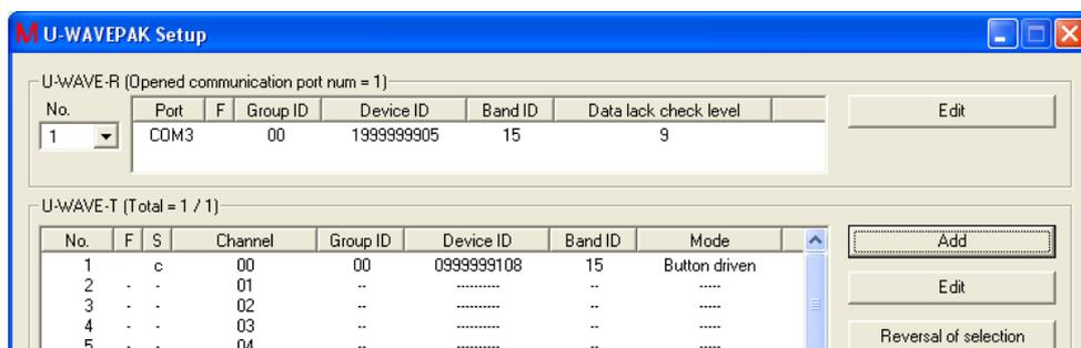
'S' row in this dialog changes from 'r' to 'c' when a wireless communication succeeds. ('c' = Wireless communication is connected.)
