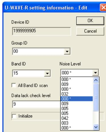
The asterisk is marked at the smallest noise level.
