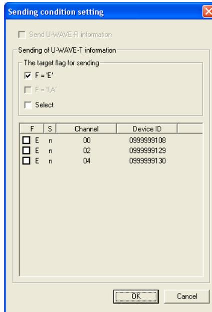
12) 'S' row in 'U-WAVE-T information' list changes to 'r' when the sending of U-WAVE-T information is completed.
