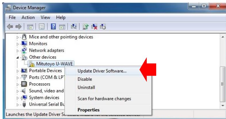
If [Mitutoyo U-WAVE] or [USB Serial Port] is not displayed in [Other devices], the device driver has already been installed. Therefore, close [Device Manager] and end the installation of the device driver.
