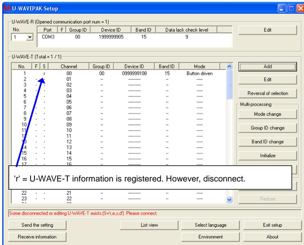
In this state, the communication by the wireless between the U-WAVE-R and the U-WAVE-T is not connected. Therefore, push an orange [DATA] switch on the U-WAVE-T once (about 1 sec) to connect a wireless communication.
