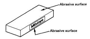
\* Attach the supplied rubber pads to the face that isn't going to be used.
