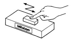
\* Minute burrs (e.g. scratches) can be removed by moving the gauge block back and forth about ten times. If there are large burrs, or when a CERA block is to be ground, apply greater pressure to the gauge block and move it to and fro as many times as required. (The size of the gauge block will not change if heavy pressure is exerted on it.)
